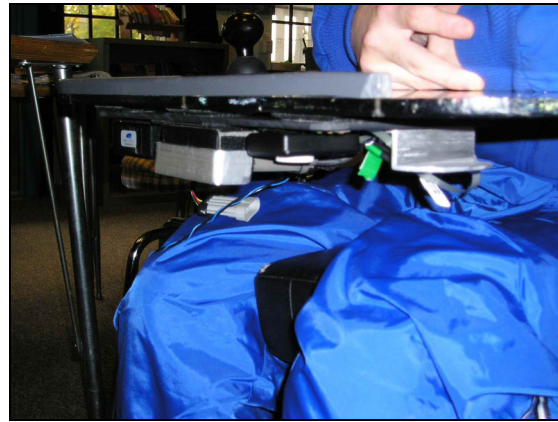
Close-up of sensing device with shield on lower half, mounted under Subject 2's lap tray.
