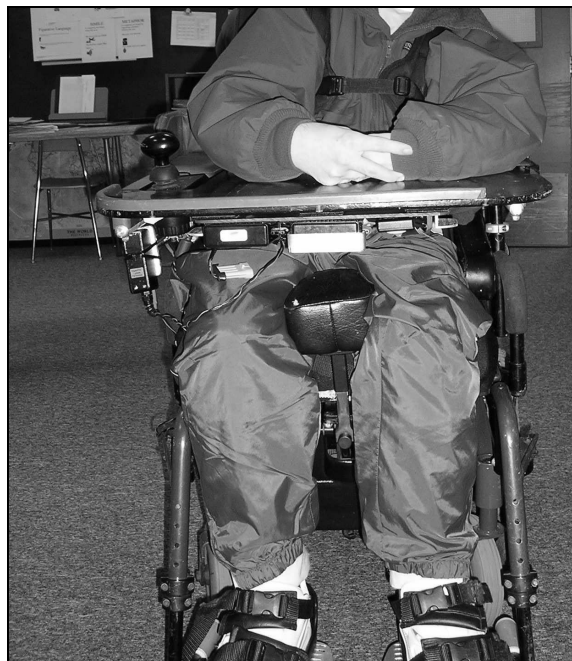
Front view of sensing device setup used in mobility training for Subject 2.
