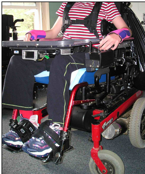
Isometric view showing Subject 1's joystick setup on her left and the sensing device mounted underneath her lap tray.
